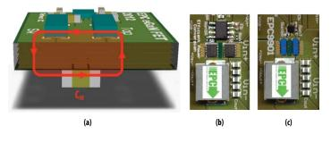
Figure 3: Conventional vertical power loop PCB layout (a) Side view (b) MOSFET top view (c) eGaN FET top view
