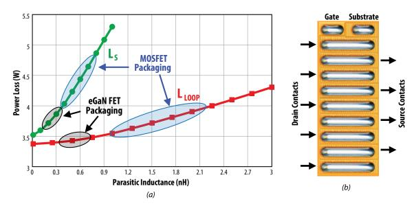
Figure 6: (a) Parasitic inductance impact on power loss ( $V_{IN} = 12 V$ ,  $V_{OUT} = 1.2 V$ ,  $I_{OUT} = 20 A$ ,  $f_{SW} = 1 MHz$ ), Top Switch: EPC2015, Synchronous Rectifier: EPC2015 (b) eGaN FET LGA package
