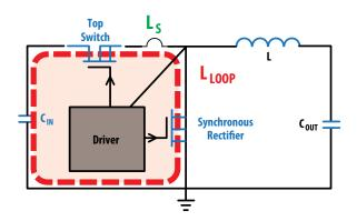
Figure 5: Synchronous buck converter with parasitic inductances
