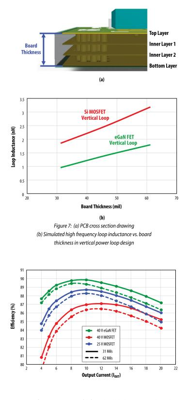
Figure 8: Efficiency comparison of different board thicknesses, 31 and 62 mils (V<sub>IN</sub>=12 V, V<sub>OUT</sub>=1.2 V, f<sub>SW</sub>=1 MHz, L<sub>BUCK</sub> = 300 nH, eGaN FETs: Top Switch: EPC2015, Synchronous Rectifier: EPC2015, 40 V MOSFETs: Top Switch: BSZ097N04LSG, Synchronous Rectifier: BSZ040N04LSG, 25 V MOSFETs: Top Switch: BSZ036NE2LS, Synchronous Rectifier: BSZ036NE2LS)
