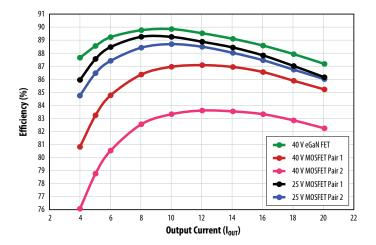
Figure 4: Efficiency comparison of 40 V eGaN FET and 40 V and 25 V Si MOSFETs at  $V_{IN}$ =12 V,  $V_{OUT}$  = 1.2 V,  $f_{SW}$ = 1 MHz,  $L_{BUCK}$  = 300 nH (Devices listed in table 1)
