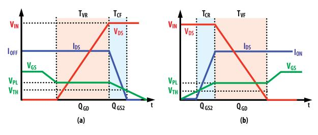
Figure 1: Ideal Hard Switching (a) Turn Off Transition (b) Turn On Transition
